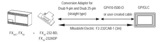
When using a CA3-CBL232/5M-01, a 9 pin <--> 25 pin conversion adaptor (straight type) is required. The FX-232CAB-1 does not require conversion adaptor and can be connected directly to PLC.
