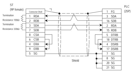
\*1 Be sure to connect the shield to the Connector Shell. For information about FG connections, refer to page 1-2 "RS422 I/F (ST400/ST403)" section's Note, in the "Connecting a Device/PLC to the ST unit."
