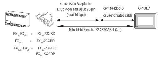
When using a CA3-CBL232/5M-01, a 9 pin <--> 25 pin conversion adaptor (straight type) is required. The FX-232CAB-1 does not require conversion adaptor and can be connected directly to PLC.
