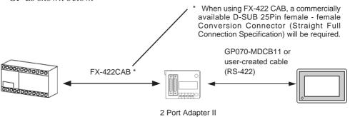
\*6 When using Digital's 2 Port Adapter II, it is necessary to connect the units to the GP as shown below.
