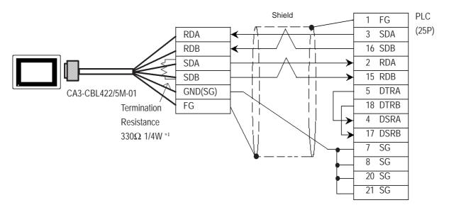
\*1 When extending the length of the cable, be sure to insert termination resistance between SDA and SDB.
