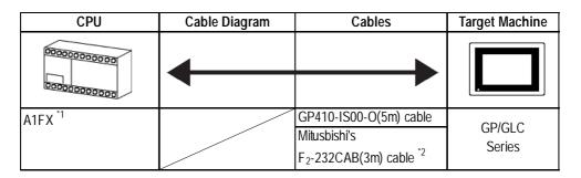
\*1 When using an A1FX, choose the MELSEC-AnN (CPU) series as the GP-PRO/PBIII project file's PLC type (refer to the MELSEC-N series manuals for the range of devices available). You will also need a 25 Pin straight cable to adjust the connector's height to align it with that of the PLC's CPU cover.
