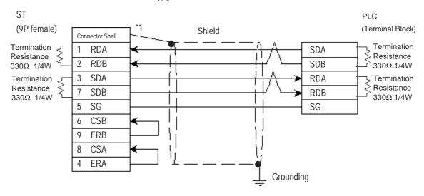
\*1 Be sure to connect the shield to the Connector Shell. For information about FG connections, refer to page 1-2 "RS422 I/F (ST400/ST403)" section's Note, in the "Connecting a Device/PLC to the ST unit."
