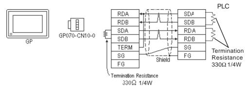
• When using Digital's RS-422 Cable, GP230-IS11-0
