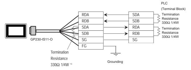
\*1 When extending the length of the cable, be sure to insert termination resistance between SDA and SDB.
