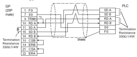
\*1 When connecting the #9 and #10 pins in the GP Serial I/F, a termination resistance of  $100\Omega$  is added between RDA and RDB.
