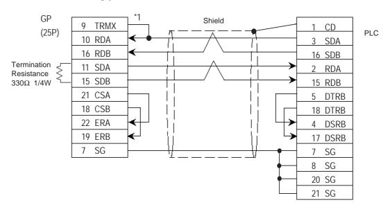
\*1 When connecting the #9 and #10 pins in the GP Serial I/F, a termination resistance of  $100\Omega$  is added between RDA and RDB.
