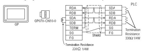
• When using Digital's RS-422 Cable, GP230-IS11-0
