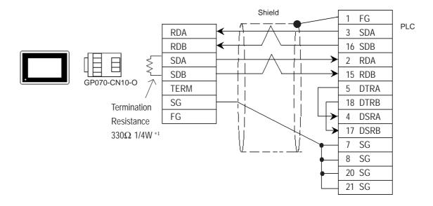
• When using Digital's RS-422 connector terminal adapter GP230-IS11-0
