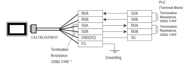
\*1 When extending the length of the cable, be sure to insert termination resistance between SDA and SDB.
