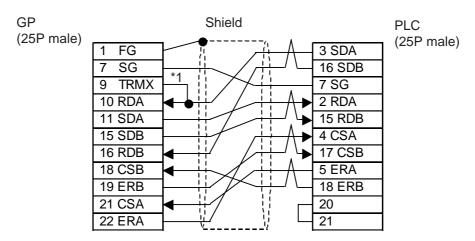
\*1 When connecting the #9 and #10 pins in the GP Serial I/F, a termination resistance of  $100\Omega$  is added between RDA and RDB.
