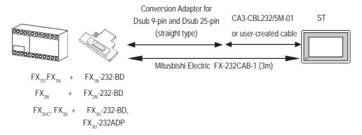
\*2 A round Dsub 8-pin to 25-pin conversion cable is required. (Mitsubishi Electronic FX-20P-CADP)
