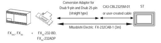
\*2 A round Dsub 8-pin to 25-pin conversion cable is required. (Mitsubishi Electronic FX-20P-CADP)
