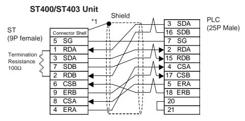
\*1 Be sure to connect the shield to the Connector Shell. For information about FG connections, refer to page 1-2 "RS422 I/F (ST400/ST403)" section's Note, in the "Connecting a Device/PLC to the ST unit."
