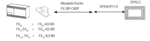
\*3 When connecting to an FX3UC, use a Mitsubishi Electric FX-422CAB0 cable to connect the FX3U-422-BD adaptor and the Interface Unit.
